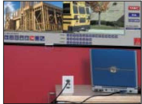
Converged faceplates and connectors allow owners to use the same faceplate for data and video connections.
