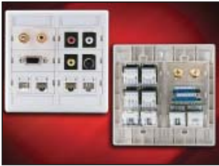
This view of a double-gang, converged faceplate details the connectors on the front that the user sees, and the actual cable interface on the back. This could be used to connect a teacher station equipped with a PC and VCR/DVD player to a projector and speakers in the ceiling.
