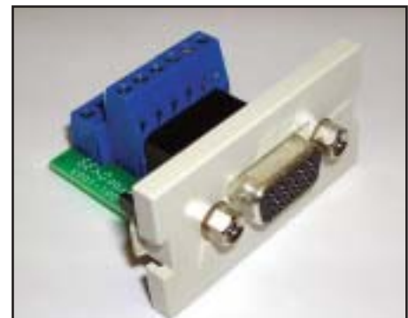
The snap-in VGA connector provides a standard HD-15 pin connector on the front, while providing an easy-to-terminate screw-down connector on the back for connection to a five-strand mini coax cable.
